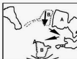
( 3 ) Black marble of Kani Khan showing difused boundary (A) between the background and calcite fractures filling as a result of homogization during Metamorphism. Always the black background is more susceptible to deformation due to impurities content. The photo and diagram below show the flow of the black background as indicated by arrows. This cause detaching of a piece (B) from main white calcite fragment (C), after the detaching the piece is rotated 180 degrees. The diagram only shows the central area of the photo.
