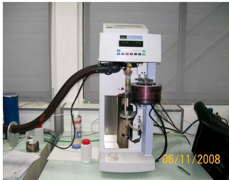
Figure (2-10): TGA analyzer type Pyris series 1 TGA.
