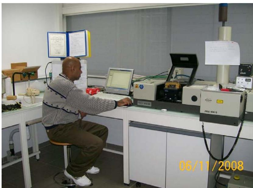
Figure (2-8): FTIR instrument type IFS 66 / 2004. In Ecole De Mines Lab. /Ales/France.
